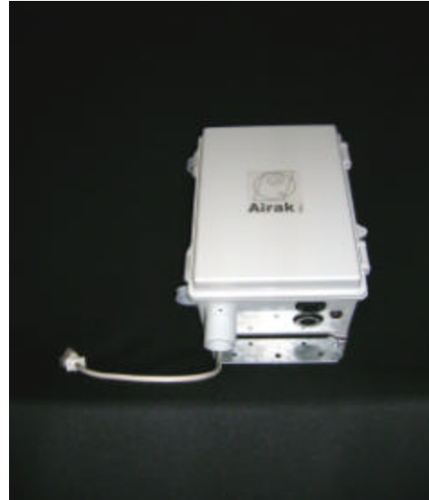
Pole mounted EOM in NEMA enclosure
